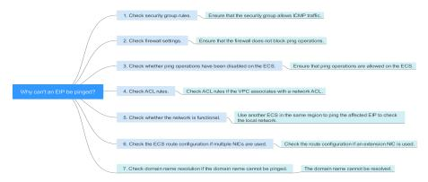
Table 5-1 Method of locating the failure to ping an EIP
